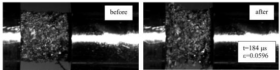
Figure 4. Failure mode at the end of the impact (strain rate =  $400 \text{ s}^{-1}$ ) - B1
