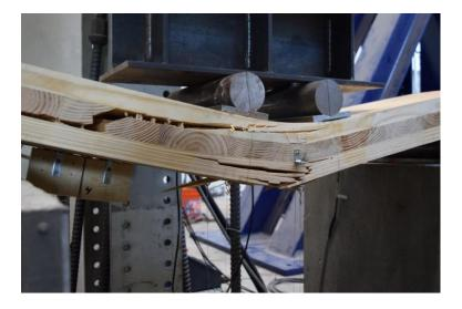
Figure 1 – CLT Beam Typical Failure Mode
