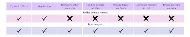
Figure 1. Comparison between the parameters involved in threat-dependent and threat-independent methodologies.
