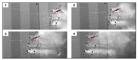
**Figure 4.** High-resolution, still-video images showing propagation of the debris field moving from right to left. The red arrows indicate potential debris breakup during the flight.
