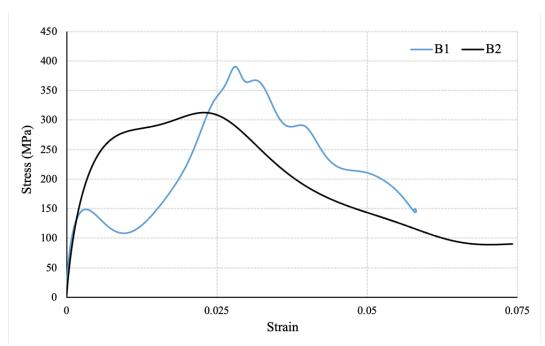
Figure 3. Stress versus strain response for BFRP bars with varying strain rates
