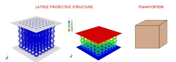
Figure 2. Representation of a lattice metamaterial and a model of a foam material
