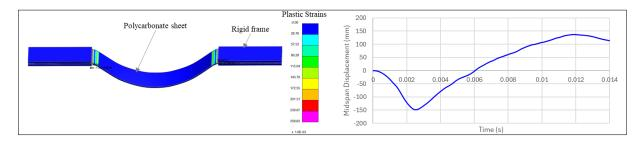
Figure 1 Deformations and plastic strains of polycarbonate sheet under blast loading (in LS-DYNA)
