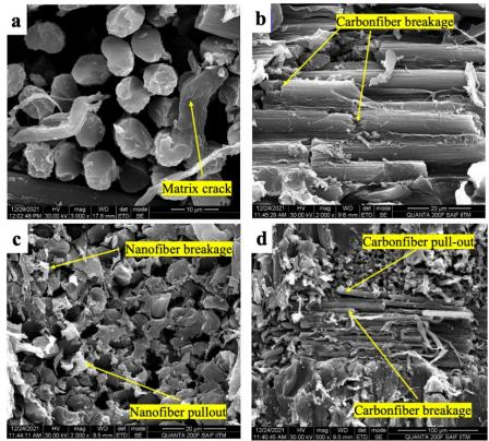
**Figure 1.** Scanning Electron Microscopy images obtained for the (**a**,**b**) CFRP and (**c**,**d**) CFRP-Nano composite
