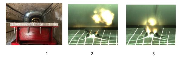
Figure 1. Video frames of the steel sandwich panel before the explosion and at different points in time after detonation. 1 - before the explosion, 2 - 468  $\mu$ s after detonation (through hole formation), 3 - 1092  $\mu$ s after detonation (ejection of fragments)
