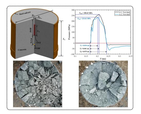
Fig 1. Damage of concrete targets and stress waves in concrete
