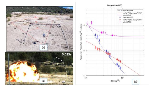
Figure 1. Experimental setup, high-speed camera image, shock wave parameters compared to TNT (UFC 3-340)
