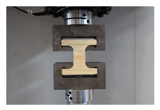
Figure 2 – Quasi-Static Tension Testing of Wood Samples Perpendicular to Grain
