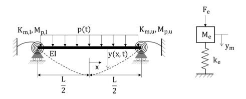
Figure 1 Equivalent single degree of freedom model for precast prestressed element with generalized support conditions
