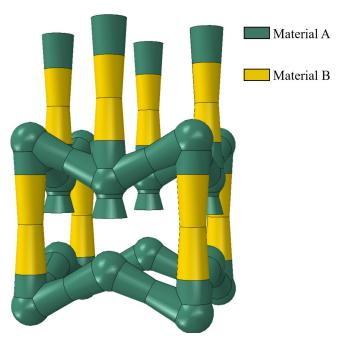
**Figure 1**: Schematic unit cell of a 3D modified auxetic re-entrant honeycomb utilizing a multi-material approach with two different materials.
