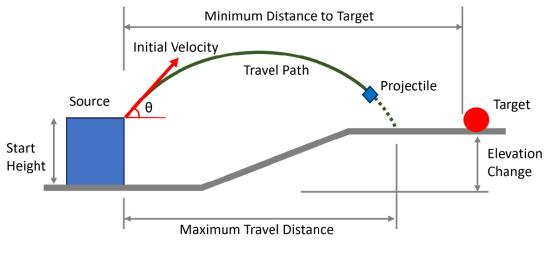
Figure 1. Projectile Motion
