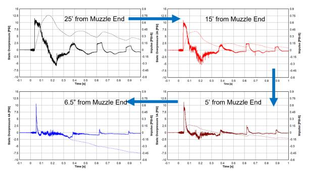
Figure 2(a). Blast wave propagation inside the driven section of MSST.
