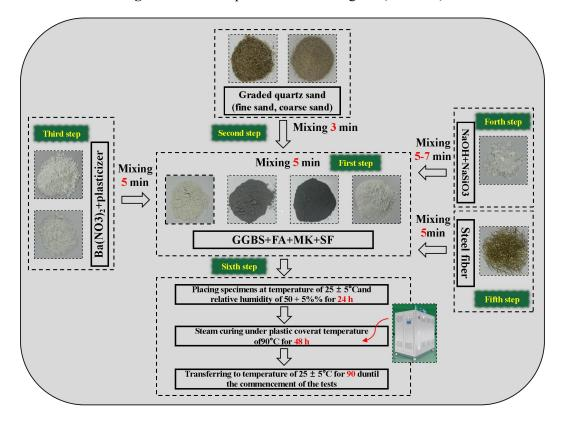
Fig. 2. preparation flow chart of G-UHPC
