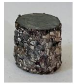
Figure 2. BFRP bar sample
