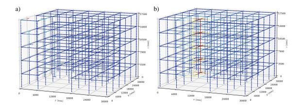
Figure 2: Progressive collapse assessment of a frame structure subjected to the loss of multiple columns. (a) Initial damage state. (b) Final damage state
