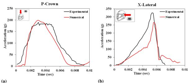
Figure 5. Acceleration history comparison between experimental and numerical simulations for (a) crown and (b) lateral impact.
