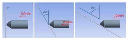
Figure 1. Projectile-specimen configuration for numerical model
