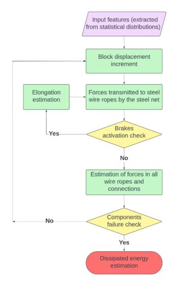
Figure 2 – Process used in the global analytical model to estimate the energy absorption capacity of a generic barrier with a given service life and for a generic impact
