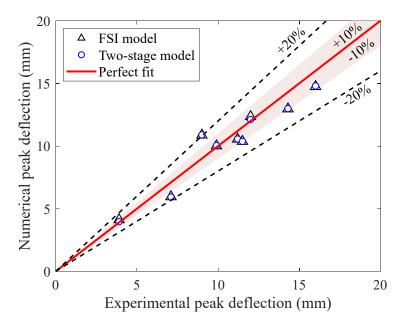
Fig. 2. Numerical and experimental values of peak deflections at the center of the steel plate
