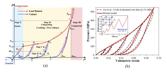
Fig.1 Equation of state and cyclic hydrostatic compression single-element test.
