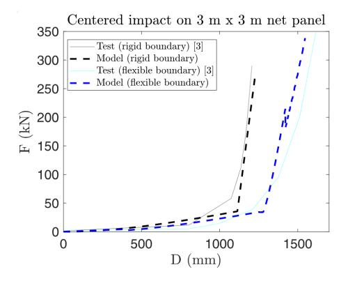
Figure 1 - Application of the fibers equivalent model to a 3 m x 3 m net panel considering ring R5/3/300: the energy dissipated by the wire ring net can be estimated by calculating the area below the load-displacement curve
