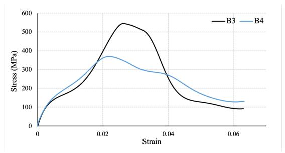
Figure 6. Stress versus strain response for BFRP bars with intermediate strain rates
