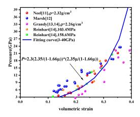
Fig. 1. G-UHPC Equation of State Diagram (3-40GPa)
