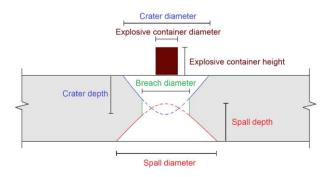
Figure 2: Representation of the failure modes on concrete slab facing a contact detonation
