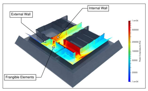
Figure 1 CFD Peak Overpressure Render
