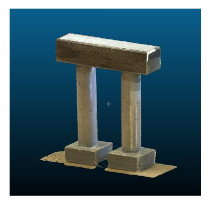
Figure 2: LiDAR-developed Point Cloud Model of an Intact, Small-Scale Bridge Pier in Cloud Compare
