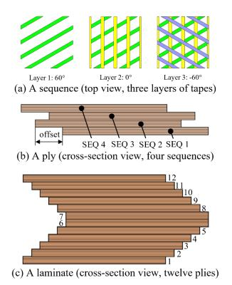
Figure 1: Layup detail of a typical interleaved composites
