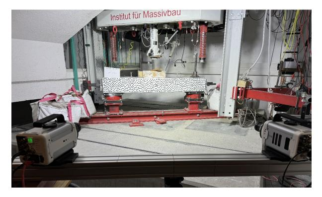
*Figure 1: Post tensioned column in the Drop Tower of TUD ready for testing. From the view-point of the high speed cameras.*
