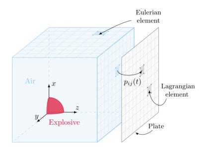
Figure 1.Uncoupled Eulerian Lagrangian approach where pressure field is mapped onto the plate.
