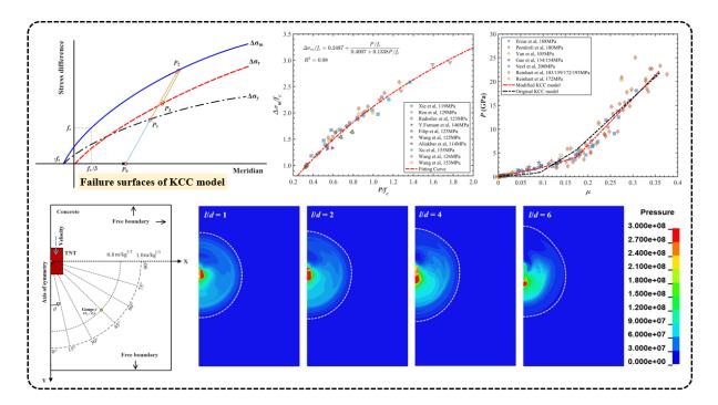
Fig 2. Calibration of parameters for the KCC model and pressure contours at 0.149 ms with different aspect ratios
