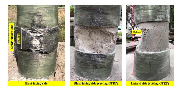
Figure 2. Failure modes of GFRP-DSTC (scaled distance=0.30 m/kg<sup>1/3</sup>)
