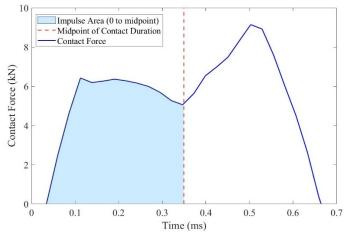
Figure 3. Force-time curve for SP-8cm-T2 (5.24 m/s), with midpoint and impulse area highlighted.
