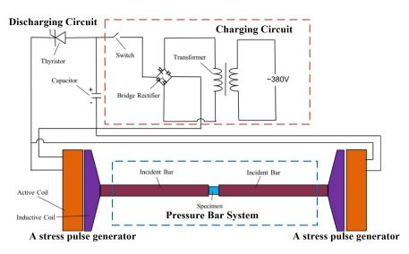
Fig. 1. Schematic diagram of the symmetric split Hopkinson compression bar
