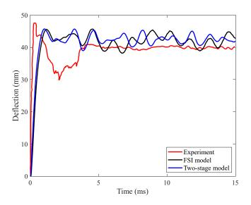
Fig. 1. Numerical and experiment results of deflection-time history at the center of the steel plate
