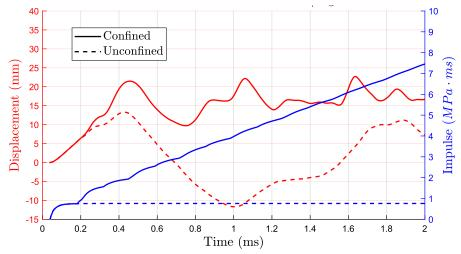
**Figure 2**. Comparison between midpoint displacement of a blast-loaded metal plates over time and impulse; two cases are reported: unconfined and fully confined blast events.
