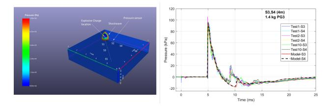
Figure 2. Simulation with Viper, Pressure signal comparison.
