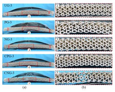
Figure 3 (a) Compress deformation of specimens with different gradient auxetic cores, and (b) enlargements of central parts of the auxetic cores.
