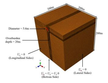
Figure 1. 3D Finite element meshed model of tunnel showing boundary conditions.
