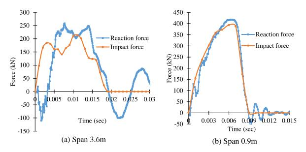
**Figure 1**. Impact force and reaction force histories for columns with span length of 3.6 m and 0.9 m
