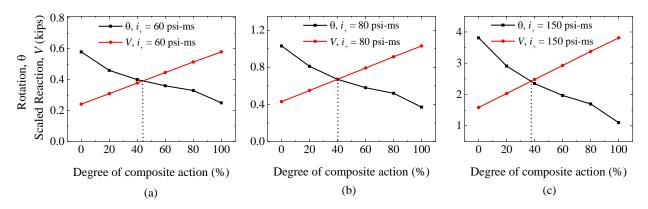
Fig 4. Variation of support rotation and scaled reactions with degree of composite action for blast impulse (a)  $i_{+} = 60$  psi-ms, (b)  $i_{+} = 80$  psi-ms, (c)  $i_{+} = 150$  psi-ms
