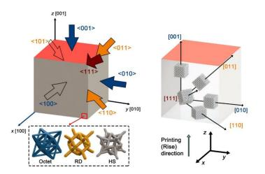
Fig. 1 Schematic diagram of lattices with different constituent cells, subjected to compression from directions other than along orthogonal axes of symmetry;
