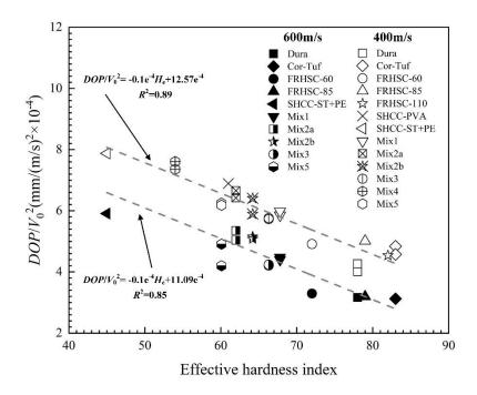
Figure 2. Normalized DOP with respect to the effective hardness index.
