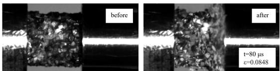
Figure 5. Failure mode at the end of the impact (strain rate =  $770 \text{ s}^{-1}$ ) - B2
