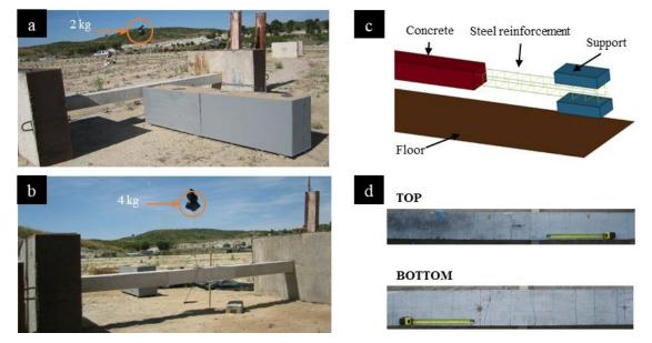
Figure 1. a) Tests with 2 TNT Eq. at 1 m distance. b) Test with 4 TNT Eq. at 1 m distance. c) Details of the numerical model. d) Results of the test b) after blast.
