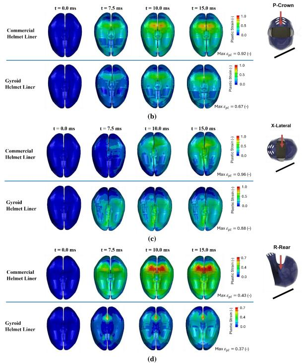
Figure 8. Fringe levels of plastic strain in the cerebrum's white and gray matter for different impact regions (a) B-Frontal, (b) P-Crown, (c) X-Lateral, and (d) R-Rear, by comparing the brain damage using the commercial EPS liner and optimised gyroid liner.
