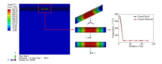
Figure 2. Temperature distribution (°C) along the tunnel at 900s.
