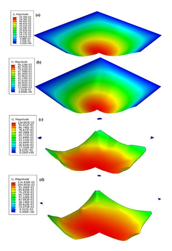
Figure 2. Deformation contours of mild steel plates subjected to underwater explosions
