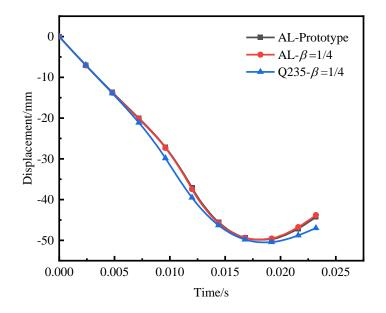
Fig. 2. Displacement time curve of curved beam.
