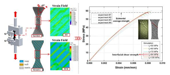
Figure 2 Method for obtaining the in-situ interfacial shear strength of 3DWCs.
