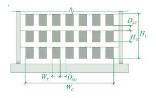
Figure 1. A schematic drawing of curtain-type blast wall
