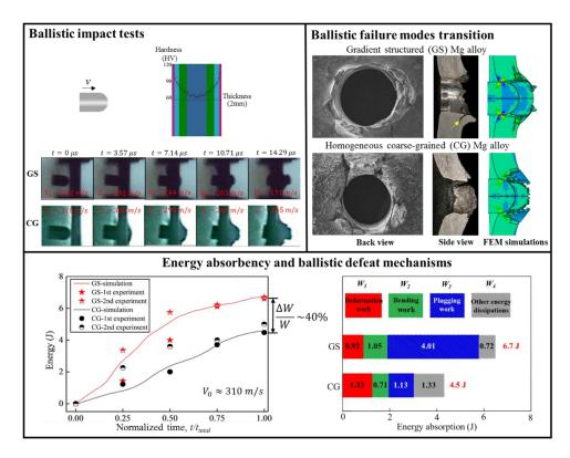
**Fig.1** The results of high-speed penetration experiments show an impressive improvement in ballistic performance due to the gradient structure design, and through systematic FEM simulations, the effects of the gradient structure on the modification of the ballistic defeat mechanisms have also been thoroughly understood.
