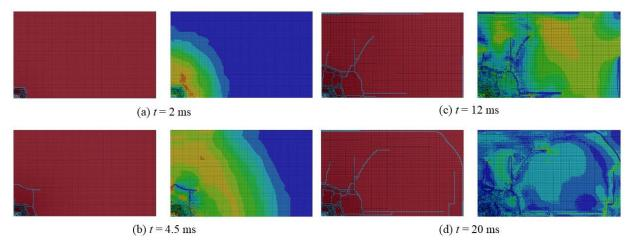
Figure 2. Glass cracking process and stress distribution
