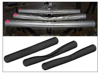
Figure 22: Comparison of simulation (left) and test (right) pipe response to blast when buried in sand
