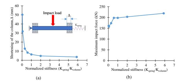
**Figure 2**. Influence of normalized spring stiffness on (a) post impact shortening of column and (b) maximum impact force resisted by column
