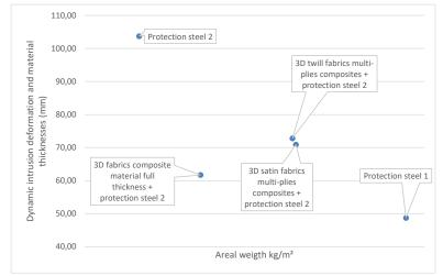
Figure 1. Comparison of different solutions submitted to explosion
