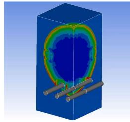
*Figure 1: Blast interaction with pipes in air simulation*
