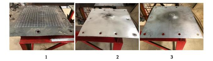
Figure 2. Photo after the explosion. Charge weight 35 gram. 1-3 mm thick steel plate (on the side opposite the explosion), 2- 10 mm thick aluminum honeycomb plate, 3- 2 mm thick steel plate (on the side of explosion)
