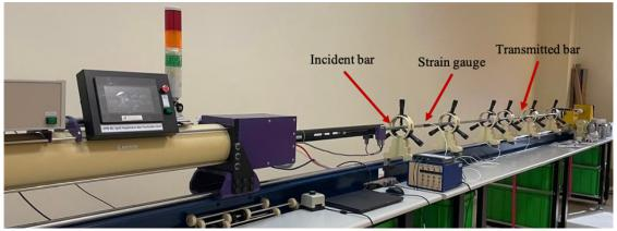
Figure 1. SHPB test set-up
