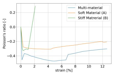
Figure 2: Poisson's ratios of the multi-material and each single material re-entrant structure.
