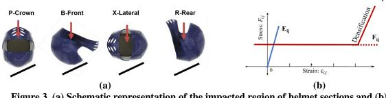
Figure 3. (a) Schematic representation of the impacted region of helmet sections and (b) Representative loading curve input for anisotropic crushable foam (MAT\_142).
