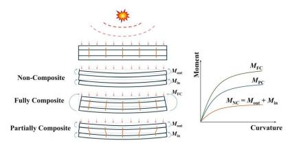
Fig 1. Behaviour of precast concrete sandwich panel under blast load
