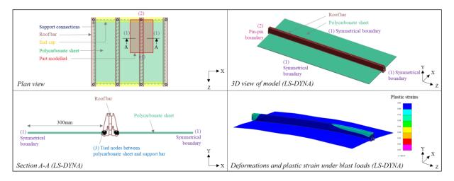
Figure 2 Numerical simulation of polycarbonate roofing system under blast loading (in LS-DYNA)
