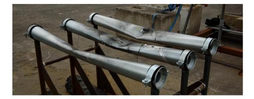
Figure 2: Air shot pipes post-firing
