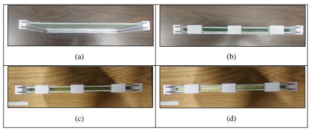
Figure (1) manufacturing steps of thermoset sandwich panel (TS-SP). (a) face sheet installation into 3D printed spacers, (b) both face sheets hold in place, (c) PU foam poured, and (d) Foam expansion.
