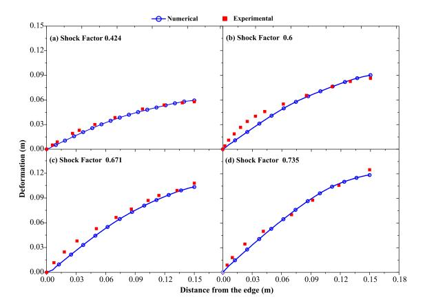
Figure 1. Validation of the present FSI model with experimental data [1] for varying SFs
