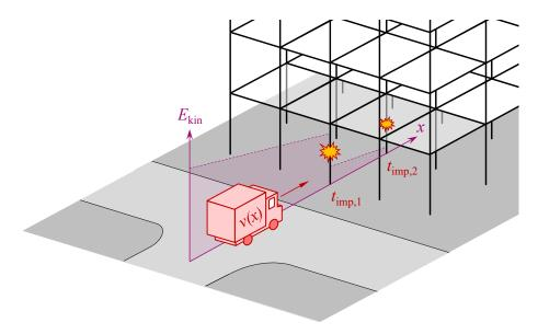
Figure 1: Time history of the kinetic energy of a vehicle for impact loading.
