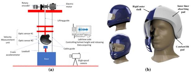
Figure 1. (a) Helmet testing machine experimental setup and (b) representative design of full-face motorcycle helmet.
