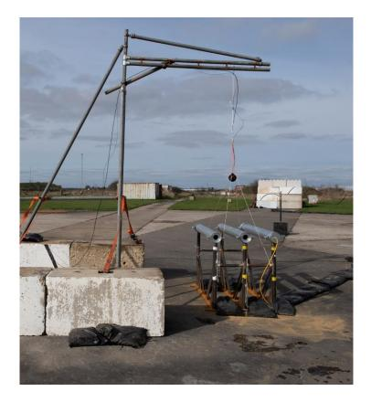
Figure 1: Air shot pipe setup pre-firing
