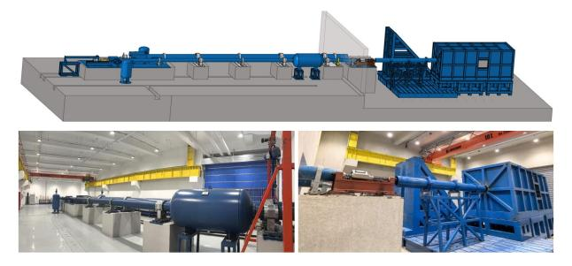
Fig. 1 Large-caliber compressive air gun in Tongji University, China
