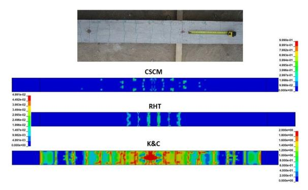
Figure 2. Field test and numerical results (LBE) of the 2 kg at 1 m distance test.
