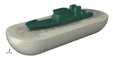
Figure 2. Example of an acoustic-structural model for UNDEX simulation in ABAQUS CAE.
