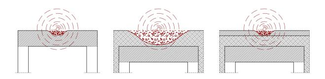
Fig. 1. Various forms of blast impact on the floor slab.
