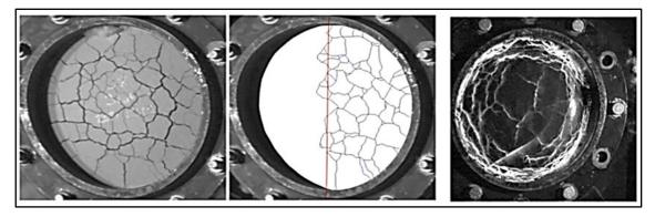
Figure 5. Images from high-speed camera footage focused on the outside face of fragmenting specimens: a 2-inch-thick concrete specimen exposed to 2240 psi (left) and a 3/8-thick glass (at 7.8 ms) exposed to 2350 psi (right).
