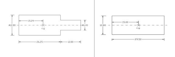
Figure 1: Schematic showing double blunt projectile design (left) with reduced primary diameter and conventional single blunt projectile (right) [2]
