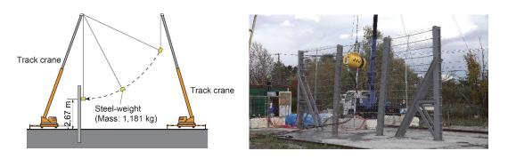
Figure 1 Setup for impact loading test. Figure 2 Deformation of fence under impact loading
