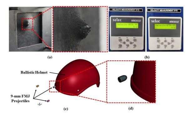
**Figure 1.** Details of Experiments and Numerical Model (a) Back Side of Composite Panel after Impact (b) Minimum and Maximum Velocities of Projectiles Impacted on the Composite Panel, and (c) Numerical Model of Ballistic Helmet Developed in LS-Dyna<sup>®</sup> for FE Simulation
