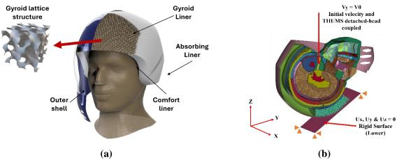
Figure 4. (a) Helmet design with exemplification of gyroid lattice structure integrated into the frontal helmet liner section and (b) cross-section THUMS head model enclosed by the commercial helmet subjected to frontal oblique impact.
