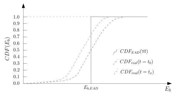
Figure 1 - Cumulative distribution functions of energy absorption for rockfall barriers: the approach currently used in the risk evaluation is graphed in black, while the expected CDF shape and its modification over time are plotted in blue and red dashed lines, respectively.
