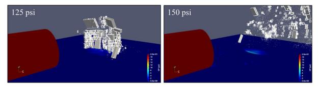
Figure 3. Coupled SHAMRC-LSDYNA calculations for 125-psi (left) and 150-psi (right) driver pressures at 149 ms.
