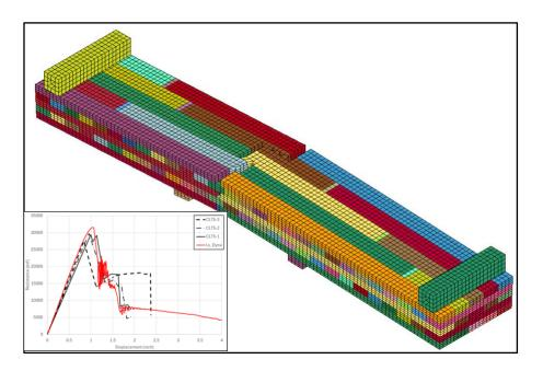
Figure 2 – CLT Beam Modeling Approach and Comparison with Test Data
