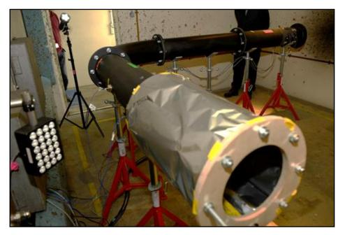
Figure 2: Setup of frangible section attachment to the Mini Air Blast Tunnel
