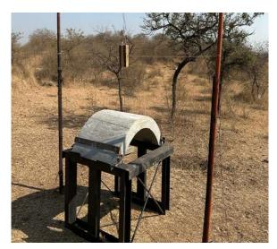
Figure 1: Curved 125 mm thick UHPFRC slab under blast load
