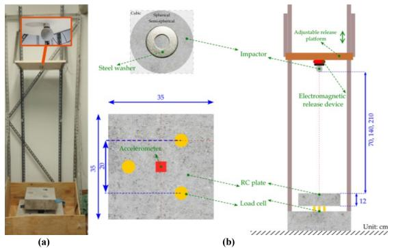
Figure 1. Experimental setup: (a) front view, (b) schematic of the experimental setup.
