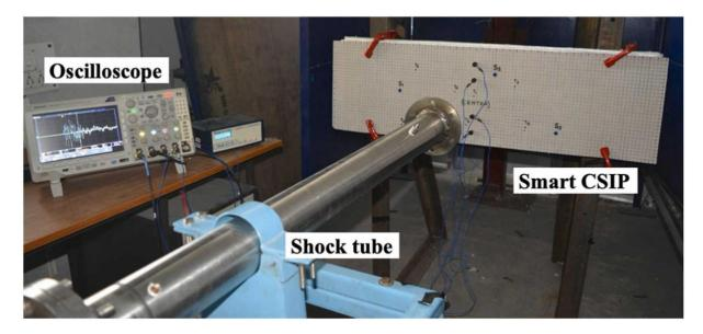
Fig 1. Experimental set up for shock tube with test specimen.
