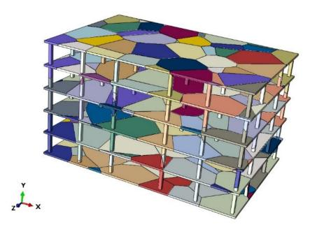
Fig. 1. Different projected debris variants using to assess ground loading
