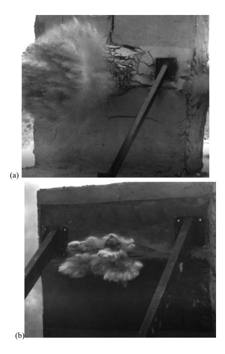
Figure 1. (a) Damage Evolution of a Masonry Wall without CFRP Reinforcement (b) Damage Evolution of Masonry wall with a single wrap of Unidirectional CFRP
