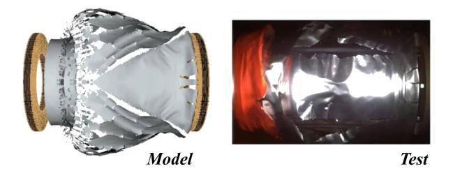
Figure 1: Model to test comparison of frangible tunnel section
