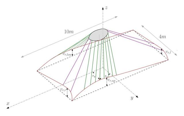
*Figure 2 – Graphic representation of the analytical model in case of eccentric impact: the displacement is imposed to the initial points of the equivalent fibers and the wire ropes deflection is calculated at each step with an iterative procedure*
