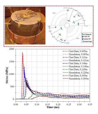
Fig.2 Simulation of stress wave propagation from spherical charge explosion in concrete.
