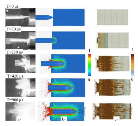
Figure 2. Comparison of test with simulation: a-Images from high speed camera, b-Simulated concrete internal strain, c-Simulated concrete external damage
