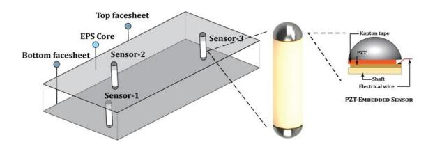
Fig 2. Detailed schematic of Smart-CSIP highlighting the sensor
