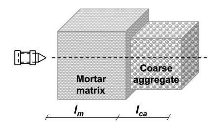
Figure 1. 1-D equivalent length assumption for the effective hardness of concrete.
