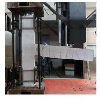
(a) RC joint with slight seismicinduced damage
