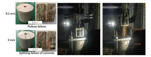
Figure 2. Dynamic pullout test and failure modes of the RC pullout specimens
