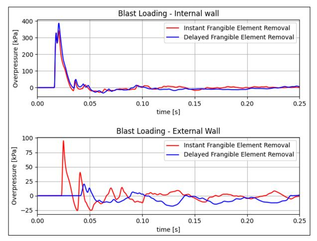
**Figure 2 Blast Loading Comparison**
