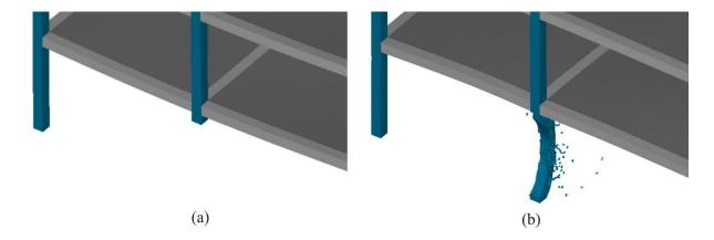
**Figure 2.** Initial damage regime for progressive collapse assessment: (a) sudden column removal, and (b) direct blast loading with 50 kg of C-4 explosive at a 1-meter standoff distance.
