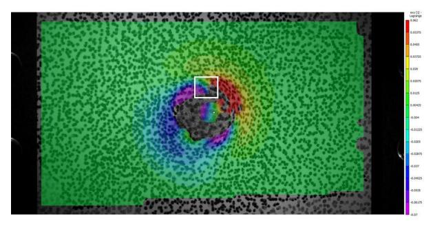
Figure 2: Shear strain contour at the capping location of an Armox 440T plate just before fracture (50 μs post detonation), the fracture initiation site is indicated by the white square.
