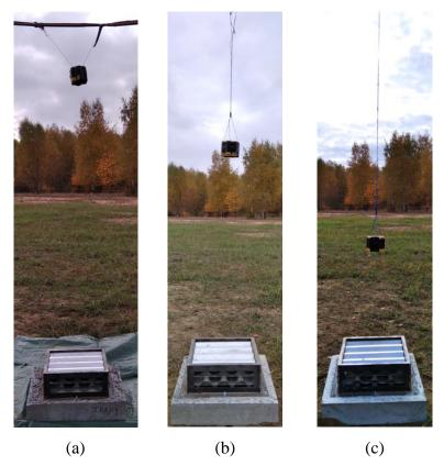
Figure 2. Distance between top layer of the blast-absorbing unit and the charge: a) H = 1.5 m, b) H = 1.0 m, c) H = 0.5 m
