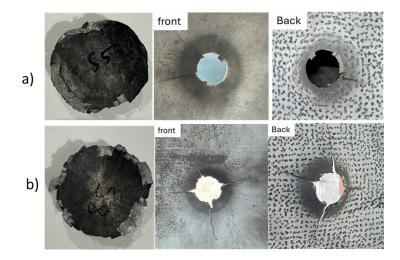
Figure 1: photographs showing the front and back views of Armox 440T plates tested at a 13 mm standoff distance with (a) 50 g and (b) 60 g PE10 cylindrical plastic explosive charges.
