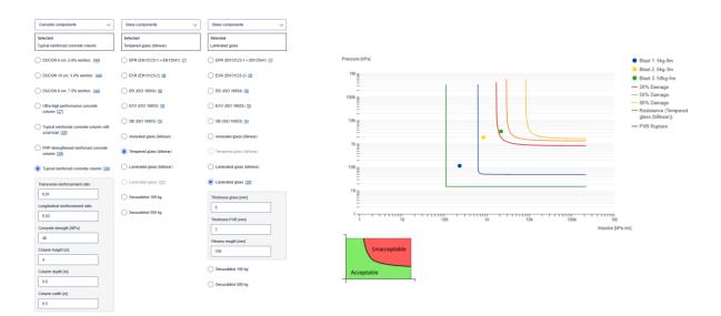
Figure 1. Selection of components and their parameters in BLADE and the resulting P-I diagram for three different blast scenarios.
