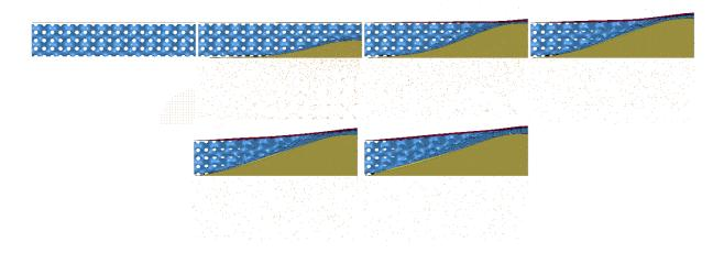
Figure 2: Deformation behaviour of TPMS filled sandwich panel (time step: 100 µs)
