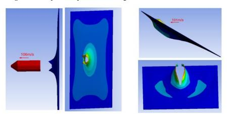
Figure 2. Numerical simulation of impact at different angles with visible change of residual velocities  $V_R$  (impact velocity  $V_0 = 120$  m/s)
