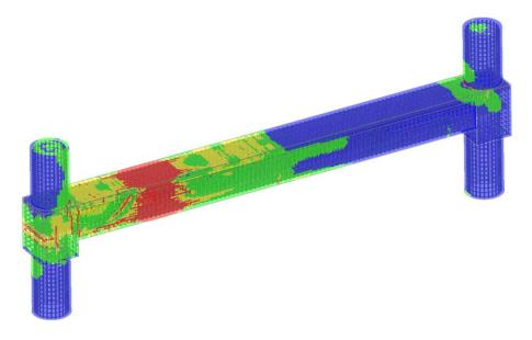
Figure 2 Full detailed precast prestressed concrete beam under close-in blast load in LS-DYNA
