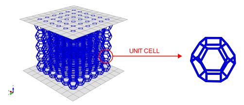
Figure 1. Lattice-based metamaterial and its unit cell
