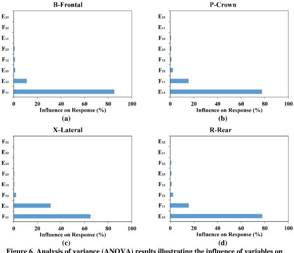
Figure 6. Analysis of variance (ANOVA) results illustrating the influence of variables on the linear approximation for different impacted regions: (a) B-Frontal, (b) P-Crown, (c) X-Lateral, and (d) R-Rear
