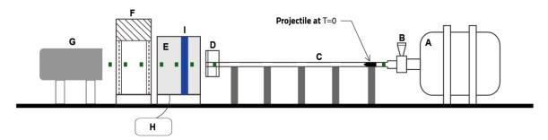
A: pneumatic chamber, B: quick valve, C: gas gun tube with supports, D: sensor to measure initial impact velocity, E: thermal chamber and specimen holder, F: sensor to measure residual velocity, G: projectile catcher, H: electronic heat controller, I: specimen – plate,  $\blacksquare$   $\blacksquare$  projectile trajectory.
