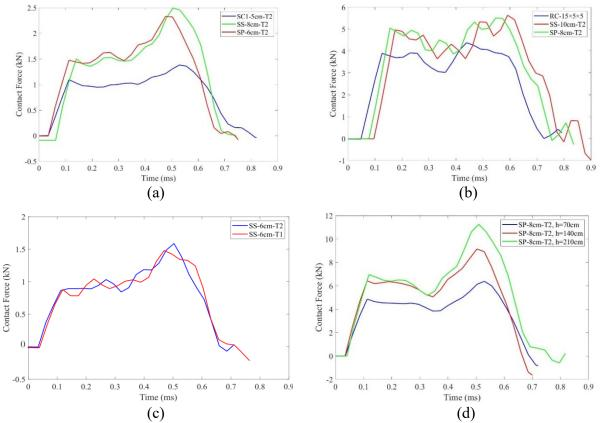
Figure 2. Time-history of contact force for samples with different: (a) contact radii, (b) shape, (c) compressive strength, and (d) impact velocity which is based on the falling height.
