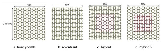
Figure 1. The geometries of the cellular metamaterials considered in this study.
