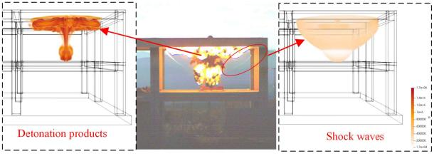
Figure 1. Comparison of the shock waves between experimental result and numerical simulation
