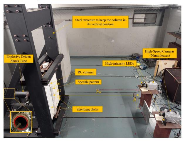
**Figure 2:** Experimental set-up for the out-of-plane displacement measurement of the columns using the digital image correlation technique.
