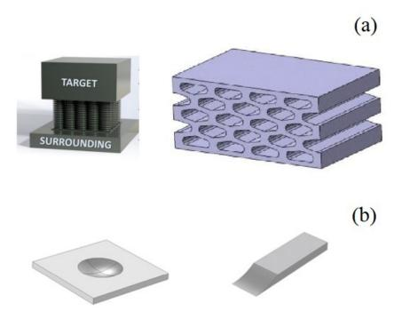
Figure 1. Examples of (a) metamaterials for vibration insulation; (b) ABH geometries.
