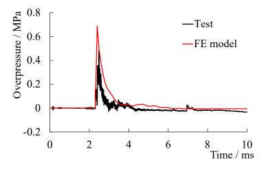
Figure 2. Comparison of the reflected overpressure time histories between experimental results and numerical simulation
