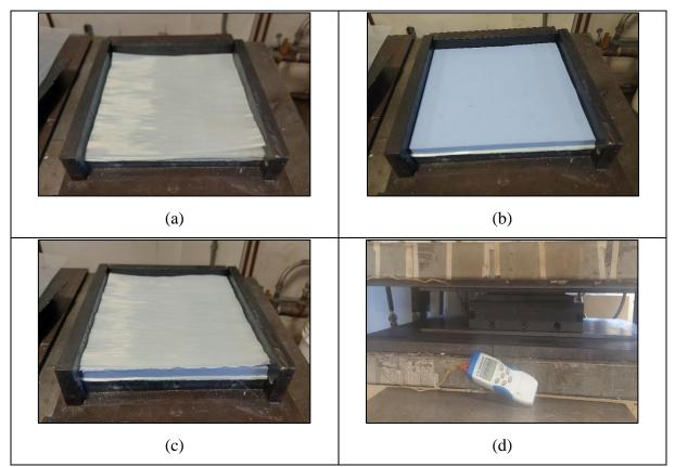
Figure (1) manufacturing steps of thermoplastic sandwich panel (TP-SP). (a) Stacking Bottom face sheet, (b) adding preformed core, (c) Stacking top face sheet, and (d) consolidating sandwich panel in press.
