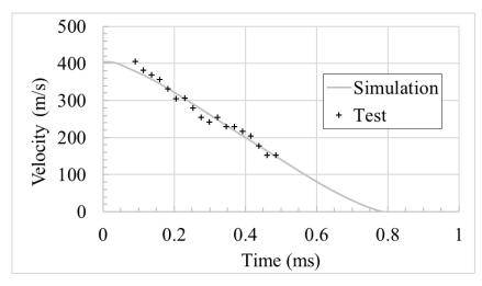
Figure 3. Projectile deceleration during penetration
