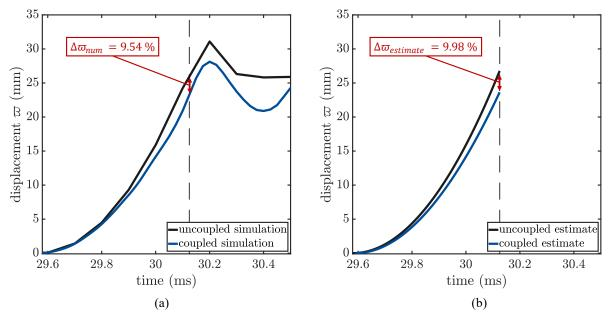
**Figure 2.** Midpoint plate deflection and dimensionless number computed from both coupled and uncoupled simulations (a), and from the analytical trends based on the uncoupled simulation (b).
