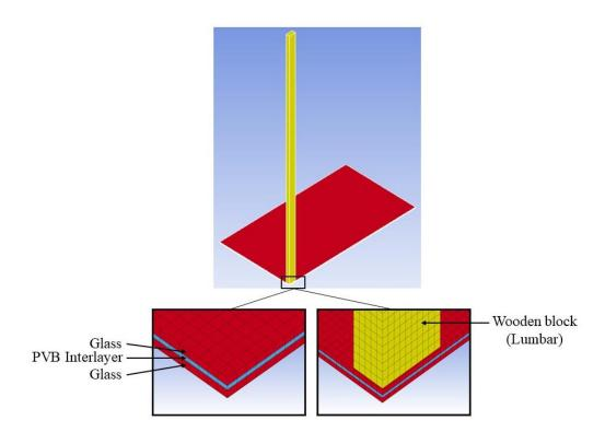
Figure 1. Numerical model of laminated glass
