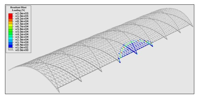
**Figure 2 FEA Blast Loading Propagation**
