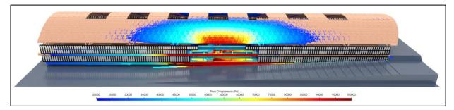
Figure 1 CFD Peak Overpressure Render
