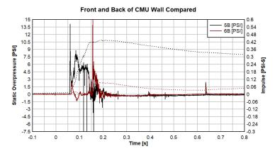
Figure 2(b). Overpressures measured in front (black) and back of (red) the CMU wall in MSST test, using transducers mounted flush in the concrete pad at the base of the wall.
