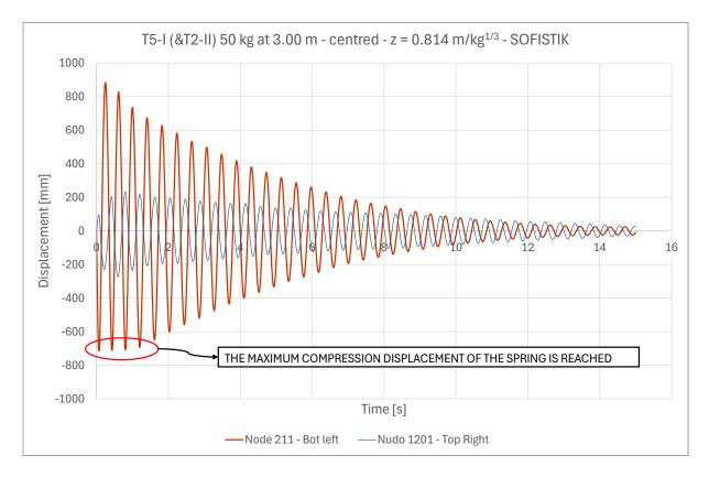
Figure 1 Displacement of bottom left and top right springs after blast
