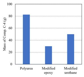
Figure 2. Fracture limit charge mass in a concrete plate 80 mm thick coated by 2 mm of resin Keywords: contact explosion, concrete plate, resin coating, spalling, fragment
