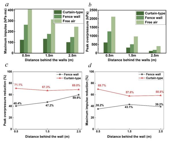
Figure 2. Comparison of blast wave attenuation effect at different gauges for three scenarios under 5 kg TNT explosion at the standoff distance of 0.4 m: (a) peak overpressure, (b) maximum impulse, (c) peak overpressure reduction, (d) maximum impulse reduction.
