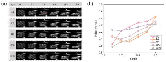
Figure 2 Deformation modes of diverse gradient hexachiral auxetics under dynamic: (a) profiles and (b) Poisson's ratio. 2. Sandwich Panels with Hexachiral Auxetic Cores Under Explosive Loading
