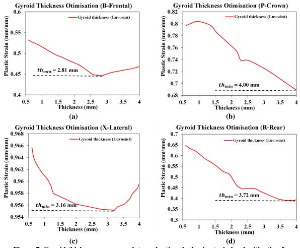
Figure 7. Gyroid thickness response plots evaluating the brain strain level mitigation for different impact regions (a) B-Frontal, (b) P-Crown, (c) X-Lateral, and (d) R-Rear.
