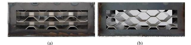
Figure 1. Blast-absorbing units: a) trapezoidal, b) hexagonal
