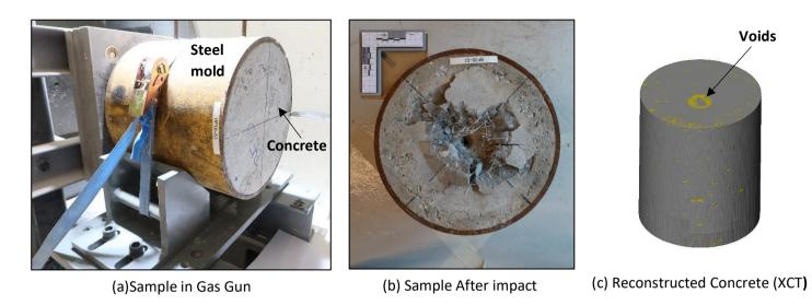
**Figure 1**. (a) sample placed inside Gas Gun Chamber with steel mold, (b) Basalt fiber sample after 12.7 AP projectile impact, and (c) Reconstructed Basalt fiber concrete using Avizo software
