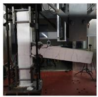
(c) RC joint with severe seismicinduced damage
