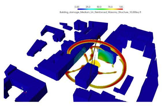
Figure 2; Example Viper::Blast analysis of surrounding Poznan city geometry.
