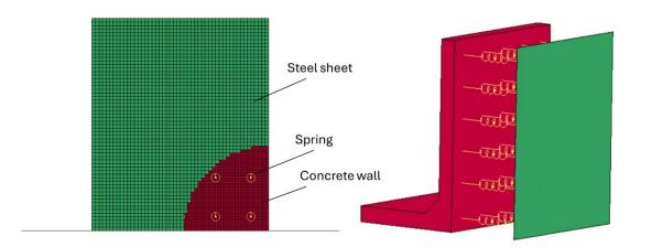
Figure 2. Numerical model of the protected wall.
