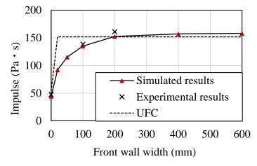
Fig.1 Effects of front wall width on blast impulse acting on front wall
